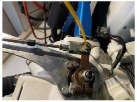
4. The seal must be passed through the hole located on the steal chainplate as shown in the photo opposite.
