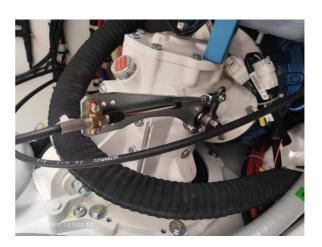
2. The Seal must be passed through the hole of 3. the upper part of the connecting rod.
